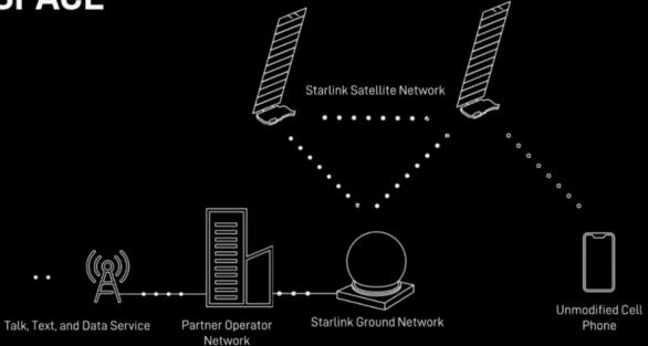
Starlink satellites with Direct to Cell capability have an advanced eNodeB modem onboard that acts like a cellphone tower in space, allowing network integration similar to a standard roaming partner.
